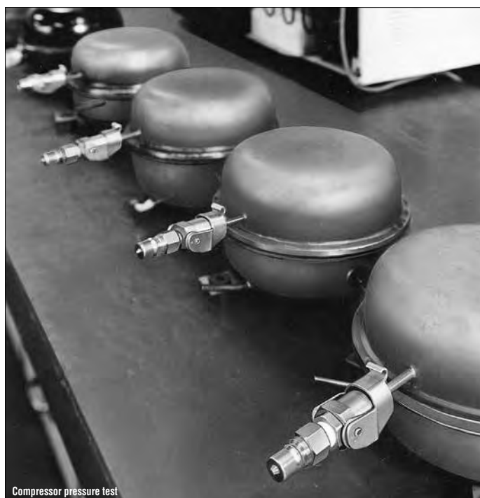
Compressor pressure test
