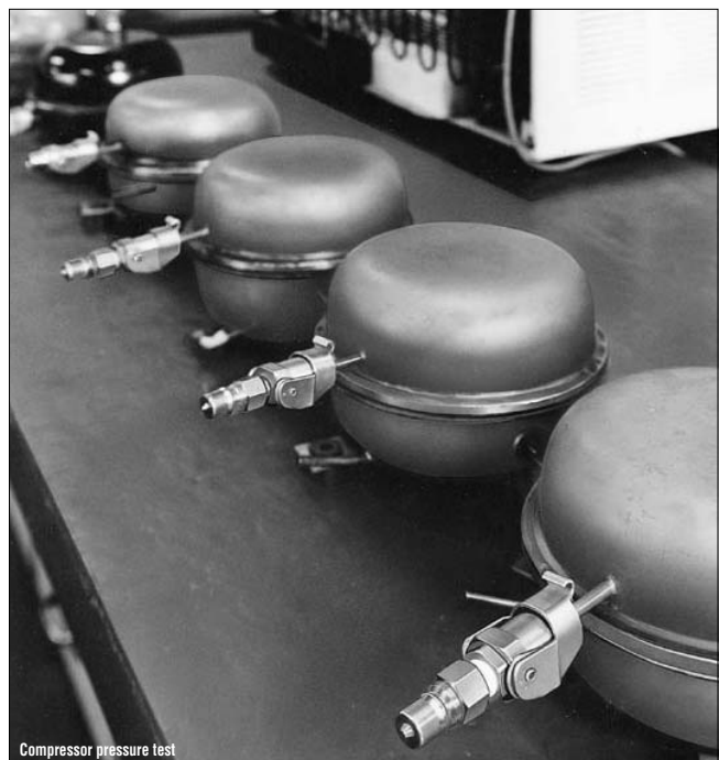
Compressor pressure test
