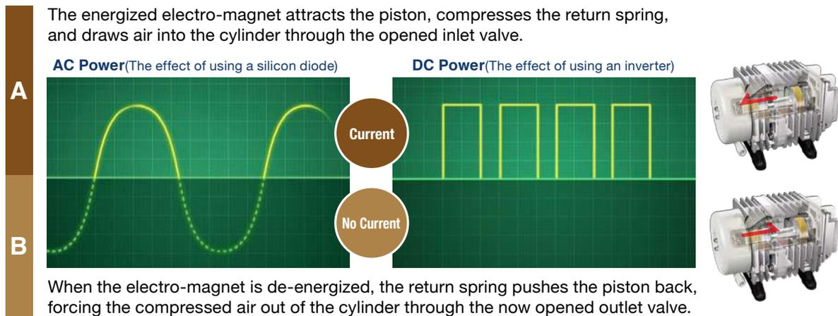
Repeating the movements of A and B delivers the function of compressor or vacuum pump.
